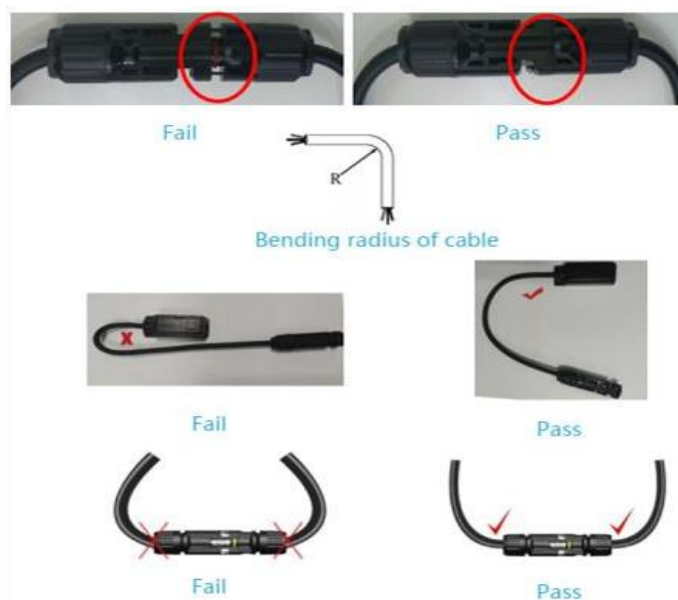
Figure 14: PV MODULES CONNECTORS
